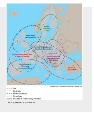
The EU has undertaken efforts to enhance energy security by enabling the import of LNG to diversify gas supply. Interconnections will be predominantly bidirectional to allow flows from both directions to be used as gas source. This is especially relevant since LNG imports typically come from different coastal areas in Europe (Figure 40) compared to the imports of gas via mainly onshore pipelines in southern and eastern EU.
