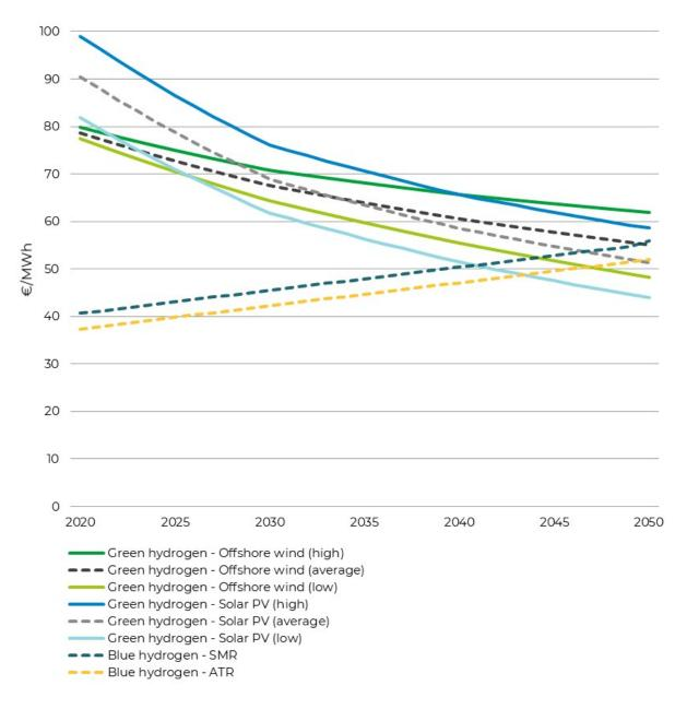
Figure 6. Development of technology costs for green and blue hydrogen in the Accelerated Decarbonisation Pathway (in €/MWh). Costs are all based on a 5% discount rate and 30-year economic lifetime.
