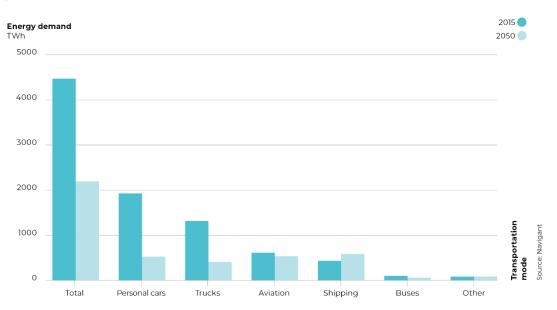
Figure 29. EU energy use in the transport sector for various subsectors in both 2015 and Gas for Climate 2050 Optimised Gas end state.
