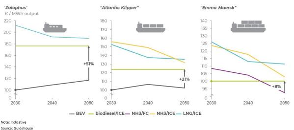
Figure 32. Lowest TCO fuel/engine combinations for three ship prototypes
